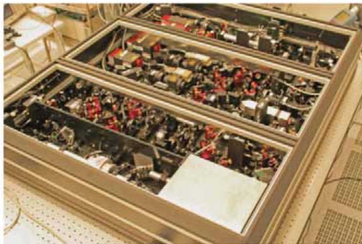
Figure 3. Photograph of the GEO600 squeezed light source. The breadboard dimensions are 135 cm x 113 cm. The three Nd:YAG Lasers are located on the upper left, at the bottom left the squeezing resonator and on the bottom right the homodyne detector with its covering box is shown. The total weight of the complete system is approximately 130 kg.
