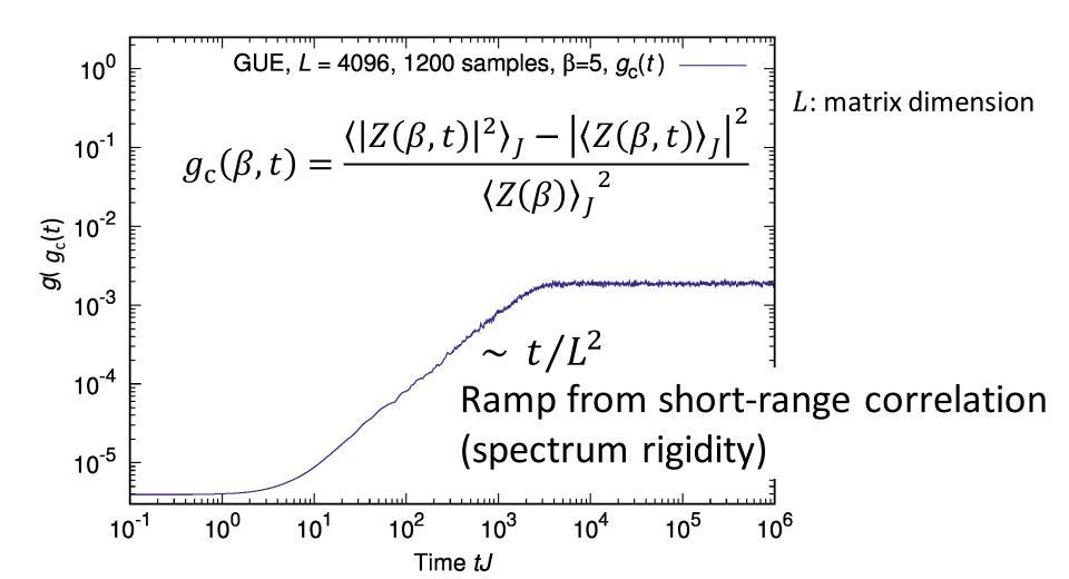
Slope-dip-ramp-plateau structure of  $g(\beta, t)$
